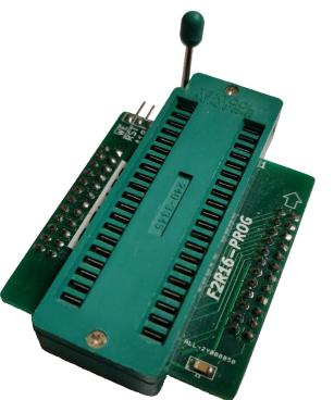
And last, the F2R16-PROG adapter from GGLabs which is used for their own nice flash ROM solution called F2R16. <u>Visit their home page how to obtain this.</u> The last step is now to combined all the adapters and the FlashROM in a stack like the picture below. Attach the correct wires from the F2R16-PROG adapter to the FlashROM. When this is ready, it's time to start the MiniPro Programmer software which comes with the TL866 universal programmer.
