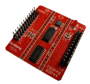
TSOP48/SOP44 Adapter from XinGong Tech is used to extend the pins and re-arange them correctly for our purpose. This can also be found of various places on the internet for a small amount of money.
