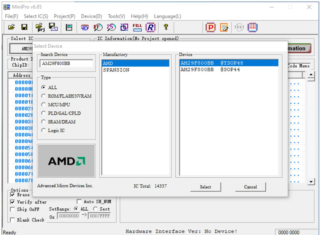
This is the basic setup to make it possible to flash and erase your FlashROM drop-in replacement for the Amiga.
