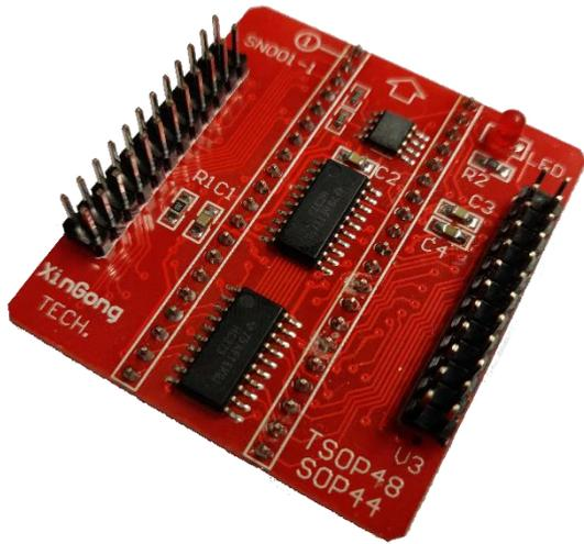
TSOP48/SOP44 Adapter from XinGong Tech is used to extend the pins and re-arrange them correctly for our purpose. This can also be found of various places on the internet for a small amount of money.
