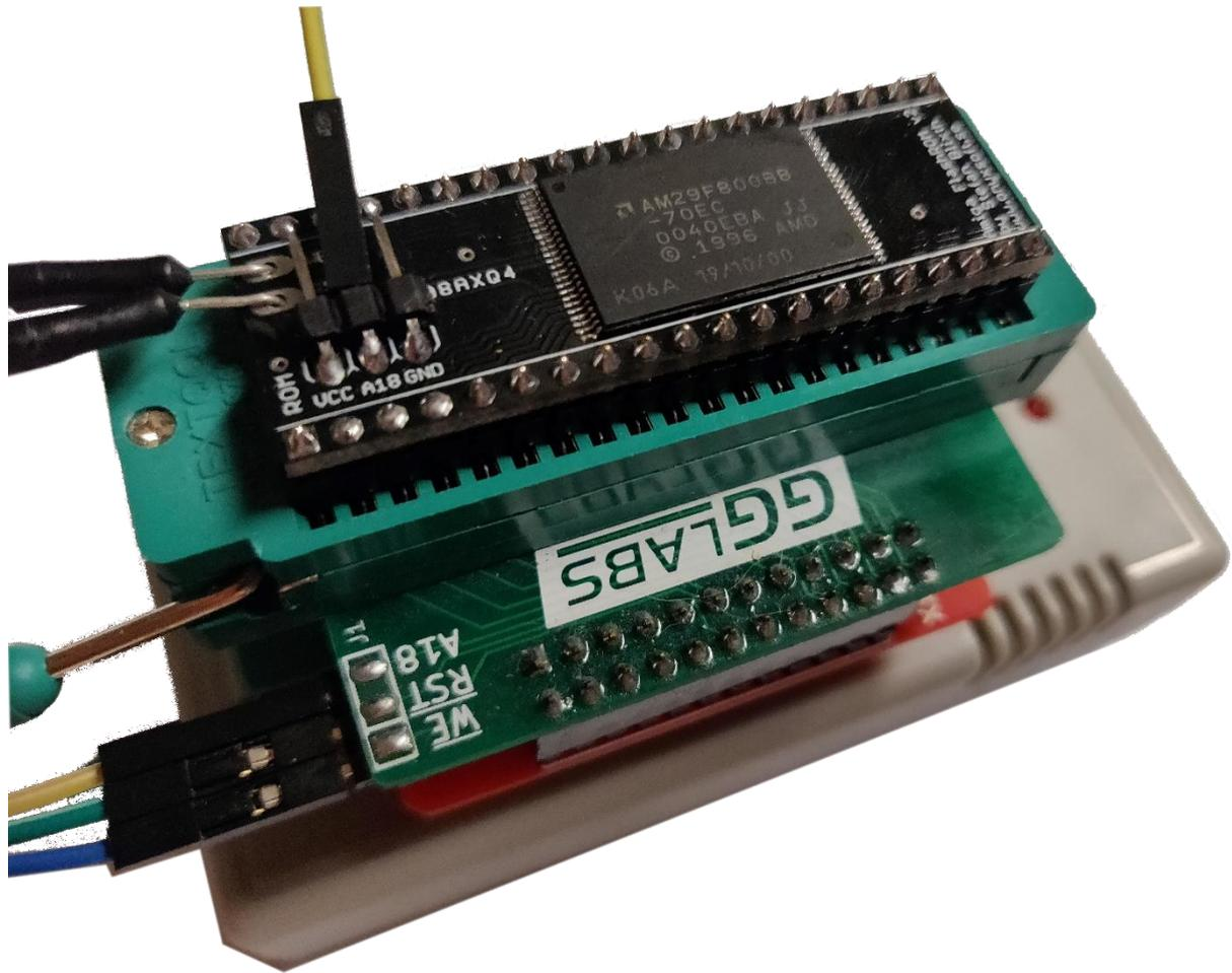
Secondly press the "Select IC" button and search for AM29F800BB as shown on the image below
